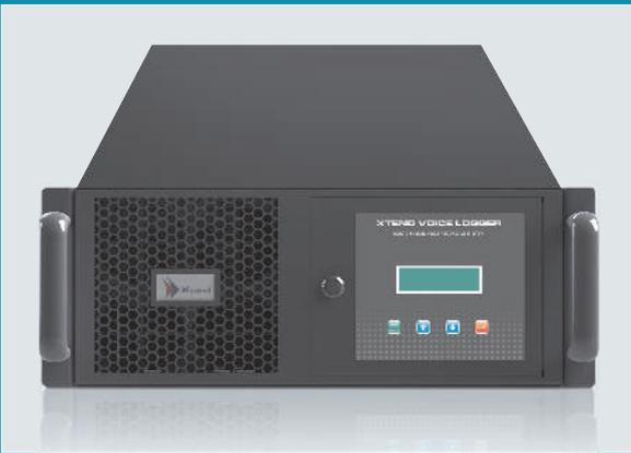
Xtend ATC Logger is a multi-channel audio/video recording solution that works with audio channels as well as analog/digital lines and RADAR. The system has the ability to capture the audio and video data during the ATC communications and can play the recordings through the browser-based user interface.
